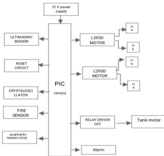
Fig.2 Block diagram pick and place
