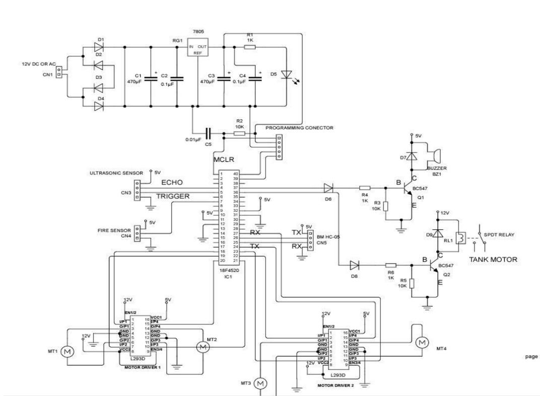
Fig.3 Circuit diagram pick and place
